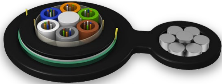
Corrugated Steel Tape Armored, Double Sheath, Figure 8 Self-supporting Cable
