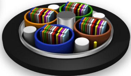
Corrugated Aluminum Tape Armored, Stranded Loose Tube Ribbon Cable
