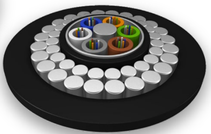
Double-layer Steel Wire Armored, Corrugated Aluminum Tape Armored, Stranded Loose Tube Cable
