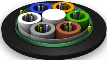
Corrugated Steel Tape Armored, Stranded Loose Tube Cable
