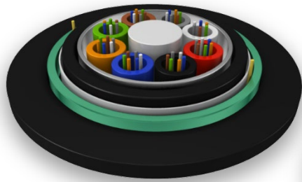
Double Armored, Double Sheath, Stranded Loose Tube Cable
