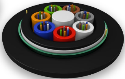
Single Armored, Double Sheath, Stranded Loose Tube Cable
